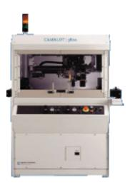
The systems utilize ball screws and servo motors (with closed-loop encoders) on all three axes to assure smooth, precise and accurate dispensing with an easy to use enhanced Graphic User Interface. These systems have been designed for the circuit board industry and use a conveyorized system to accommodate circuit boards up to 19" x 19" (483mm x 483mm) (CAMALOT 5000).
