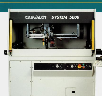
The CAM/ALOT 5000 Liquid Dispensing System provides high-speed adhesive or solder paste dispensing for applications involving large boards or multi-up panels:
